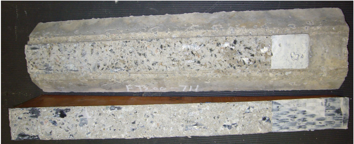
Figure B.4. Fracture of the Concrete to CFRP Interface Region – 300 Freeze/Thaw Cycles
