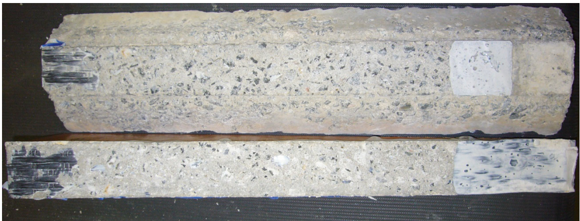
Figure B.14 Failed Interface Region of Run-out Specimen – 300 Freeze/Thaw Cycles
