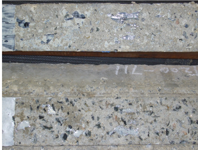
Figure B.5. Close up of Fractured Interface Region – 200 Freeze/Thaw Cycles
