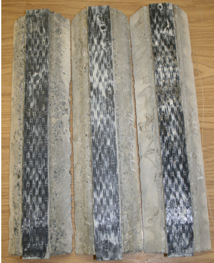
Figure B.3 Freeze/Thaw Specimens: 300 Cycles (left), 200 Cycles (center), and Pristine (right)
