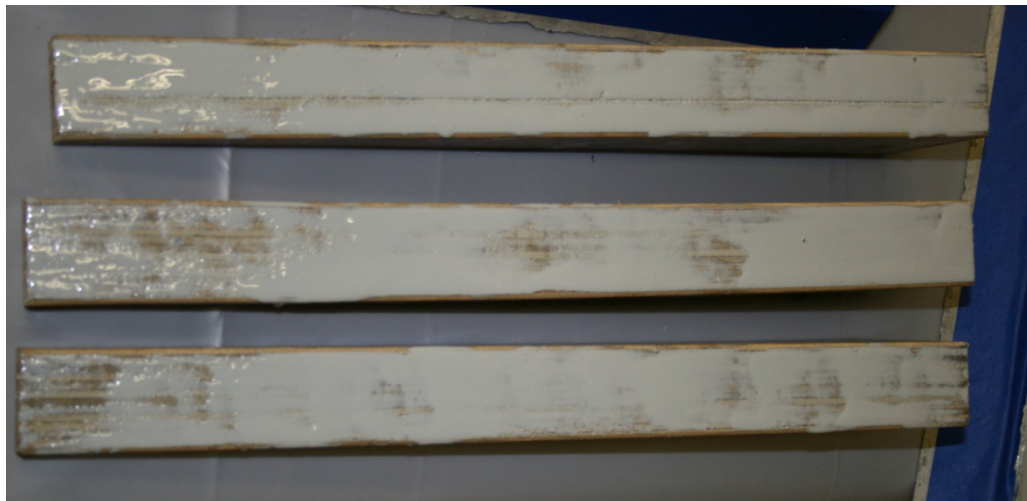
Figure B.12 Absorption of Epoxy by Microllam ® LVL
