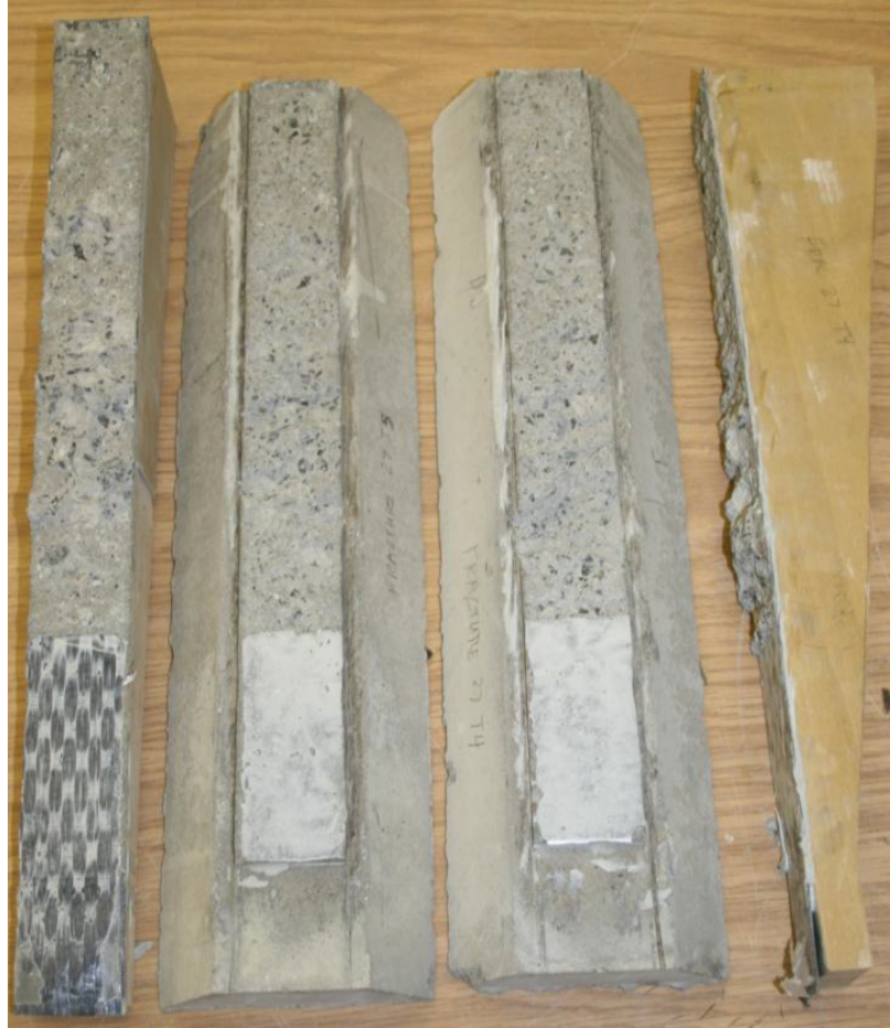
Figure 2.13 Deep Substrate Failure – FRACT27_T4 and FRACT27_T5
