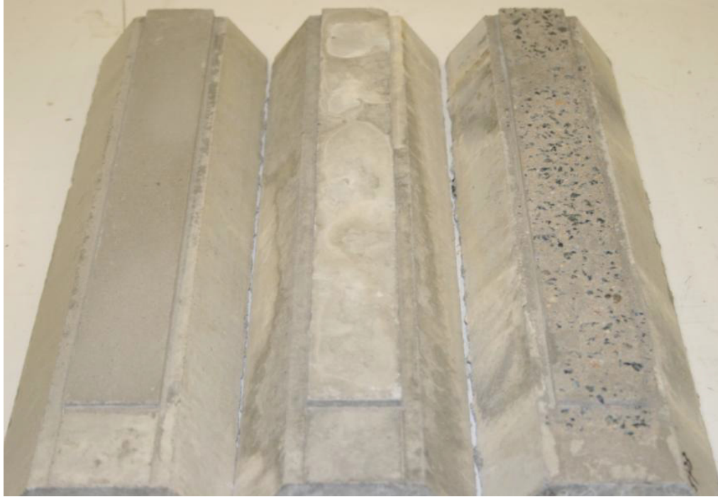
Figure 2.5 Comparison of Virgin Concrete Substrate (Center) and SP 1 Substrate (Left) and SP 3 Substrate (Right)
