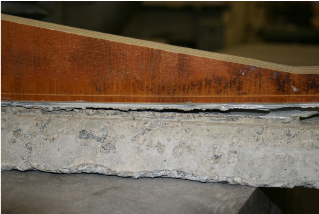
Figure B.11 Pre-Test Failure of the CFRP to Concrete Interface – 300 Freeze/Thaw Cycles
