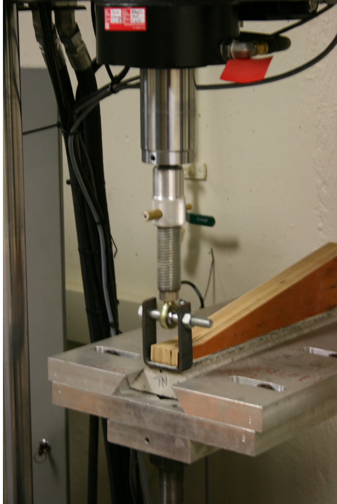
Figure 4.5 Single Contoured Cantilever Beam Fracture Test in the 20-kip MTS Machine ®
