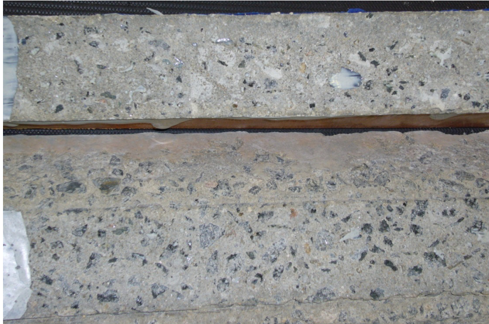
Figure B.15 Close up of Fractured Interface Region – 300 Freeze/Thaw Cycles
