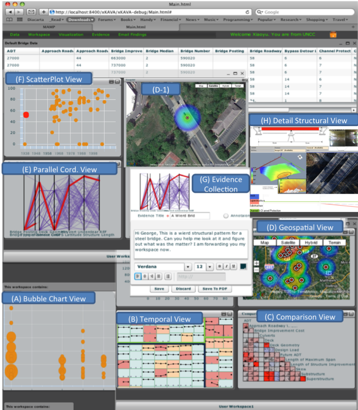
Figure 29: The overview of the entire system of iMonitor client. In this client system, iMonitor provides views for Google Map(D), Parallel Coordinates (E), Scatter Plots (F), Temporal Analysis (B), Bubble Chart (A), Comparison Matrix (C), and the original data (top row). Per-Bridge Detail View (H) and Evidence Annotation Panel(G). Several items are highlighted with colors. (D1) is used in Section 6 as part of the scenario
