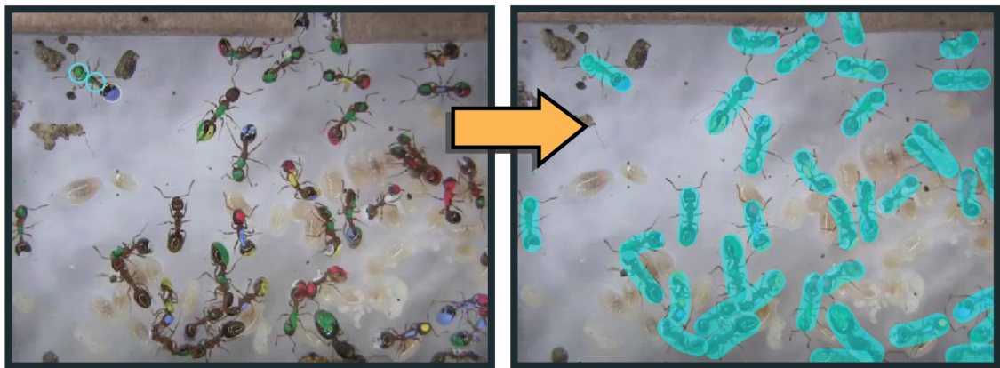
Figure 6: How the user marks the objects in a frame. Three clicks (showing the first two on the left) define the area occupied by the object. The right image shows the results of a user marking all objects in the frame. Note that overlapping marks remain separable.
