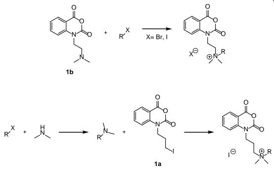
Figure 5-3: Unification of the platform onto the  $\underline{1a}$  derivative through the modification of the active halide to dimethyl amine functionality
