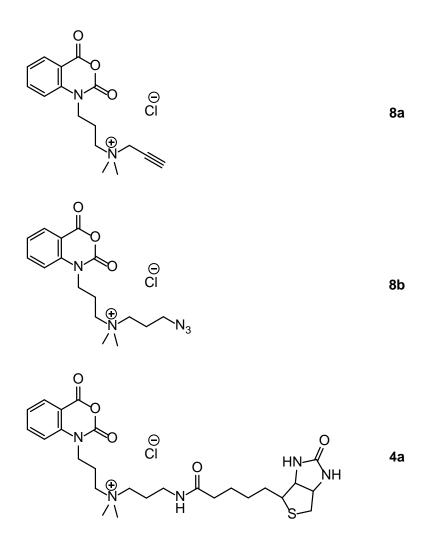
Figure 5-1: <u>8a</u>, <u>8b</u>, and <u>4a</u> isotoic anhydride derivatives used for evaluating the effects of R on the reactivity of the bioconjugate.
