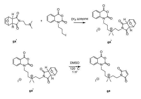
Figure 4-3: Deprotection of maleimide reagent as quaternary salt, producing heterobifunctional thiol/amine reactive reagent
