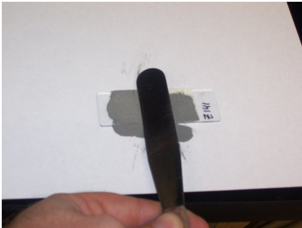
Figure 49: Applying monolayer of soil particles to slides
