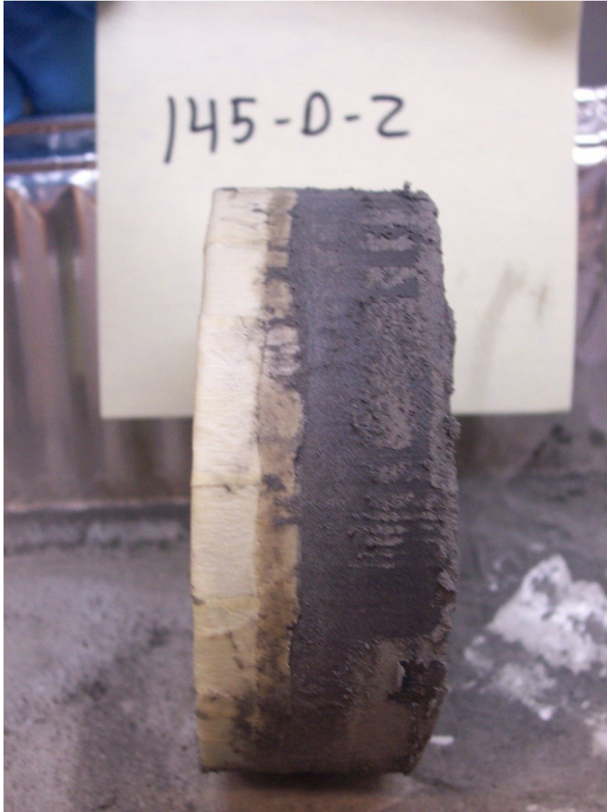
Figure 76: Confirming sample infiltration (1)
