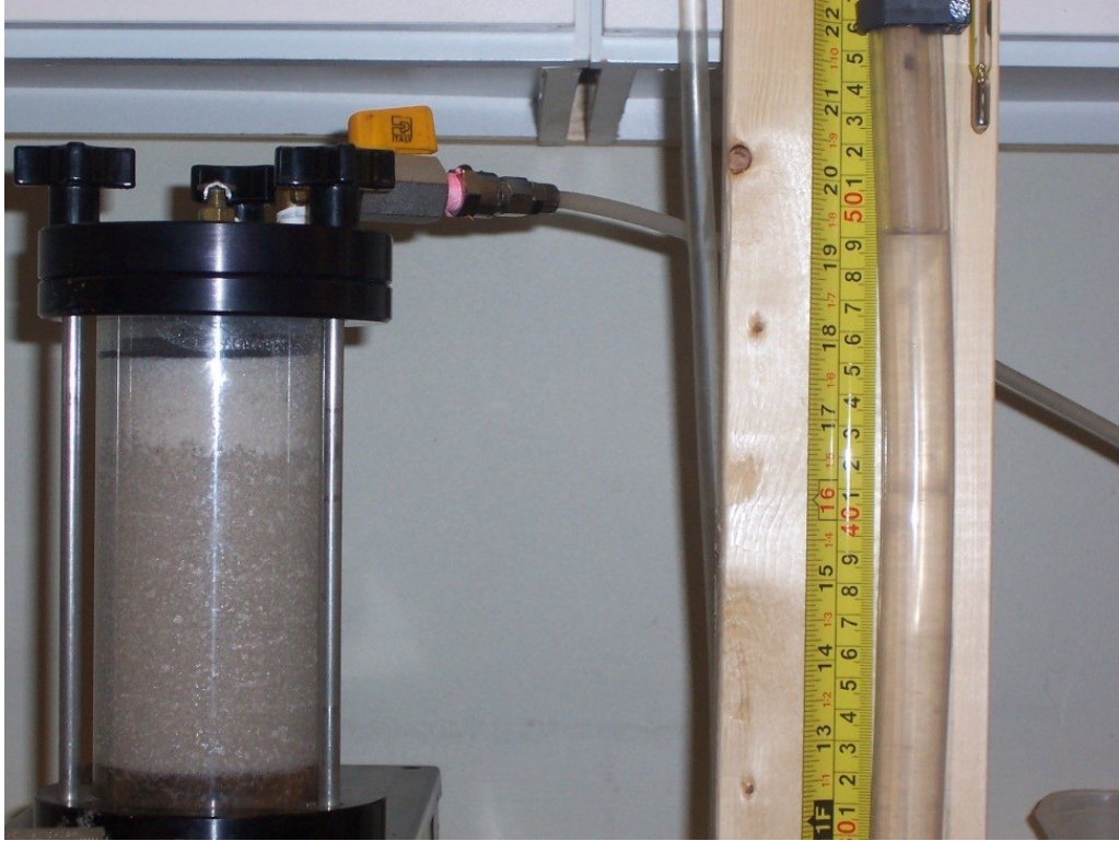
Figure 64: Hydrophobic sand in standpipe apparatus
