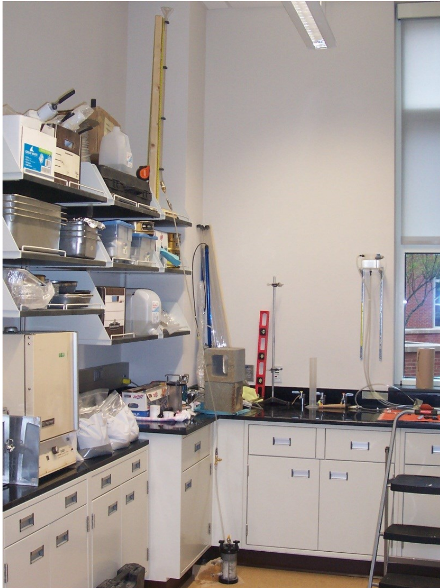
Figure 75: Standpipe apparatus with up to 3 meters of head
