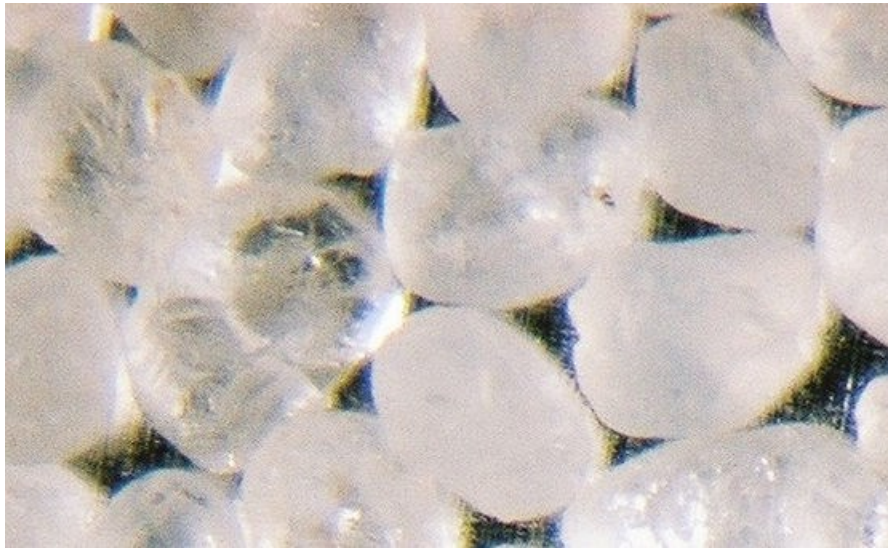
Figure 10: U.S. Silica Ottawa sand under 45X magnification
