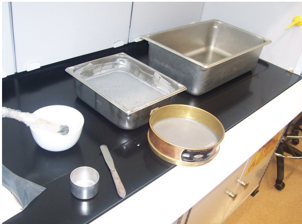
Figure 58: Equipment setup for processing treated soils
