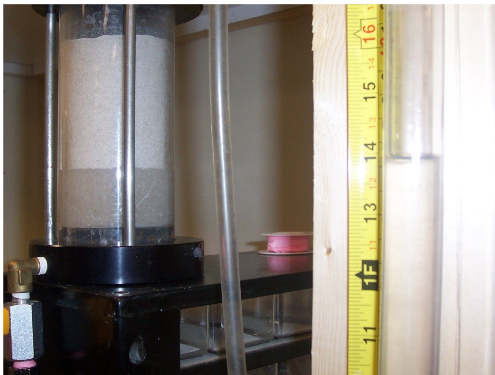
Figure 63: Hydrophilic sand in standpipe apparatus
