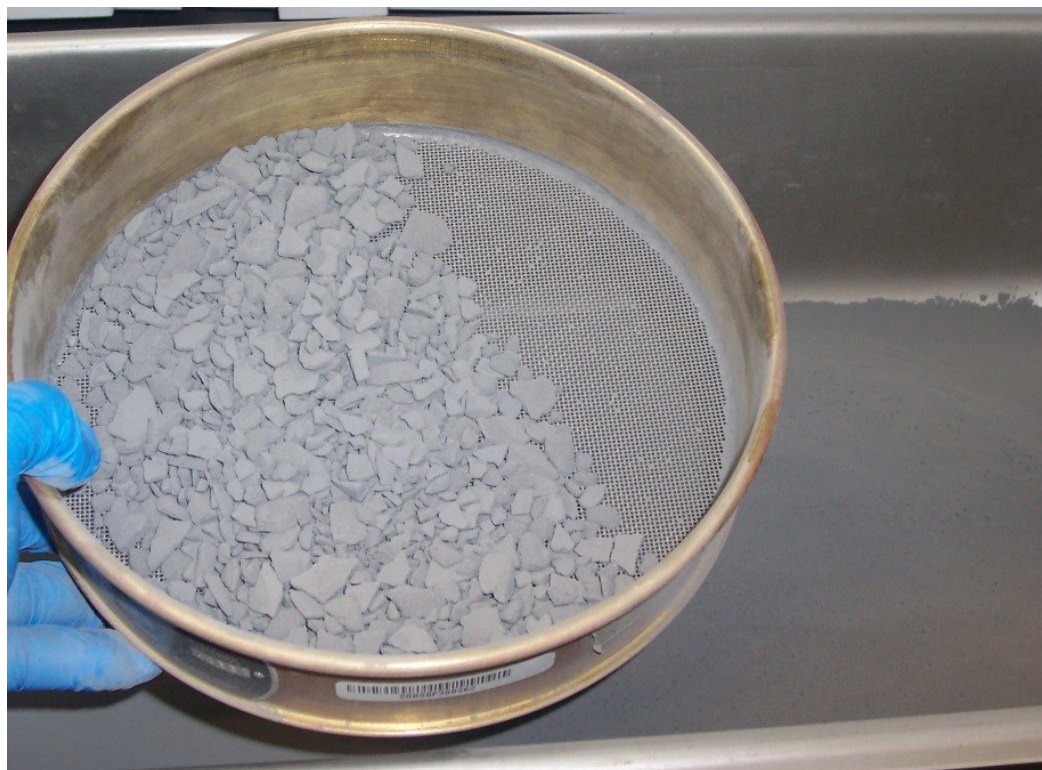
Figure 60: Passing treated CFA through #10 sieve
