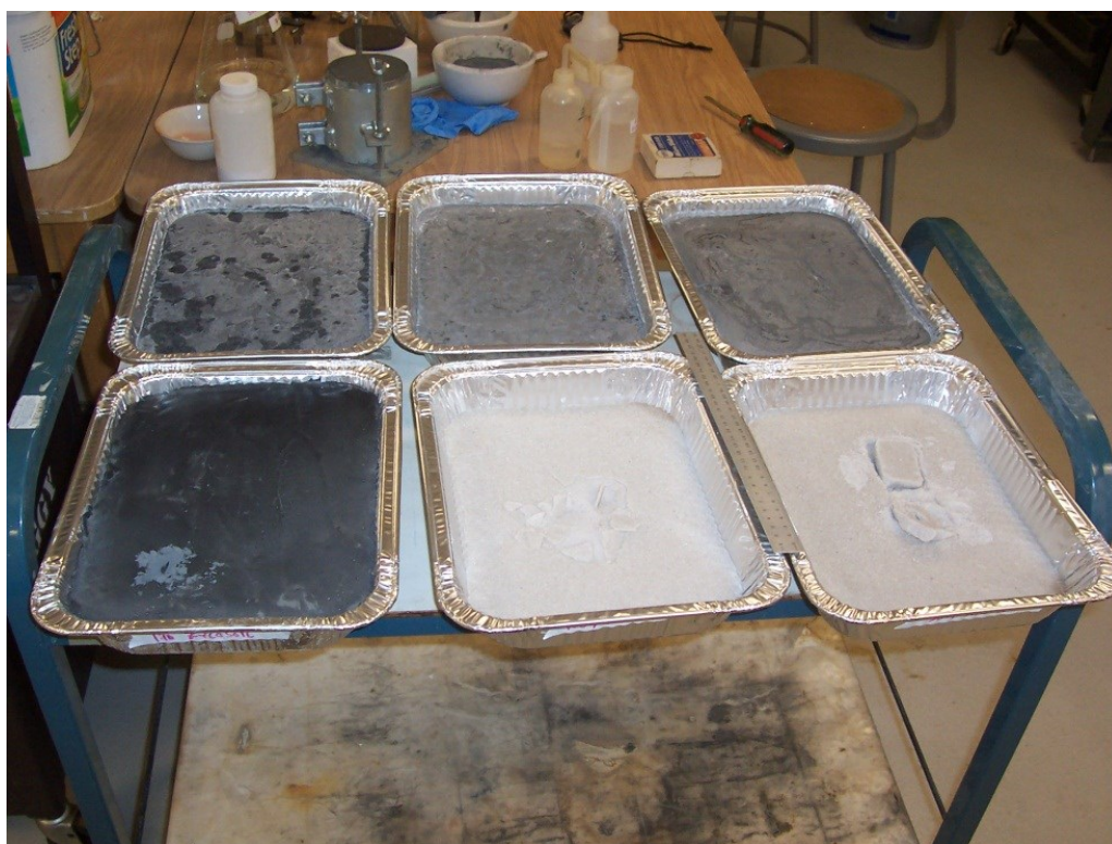
Figure 57: Large samples after oven drying
