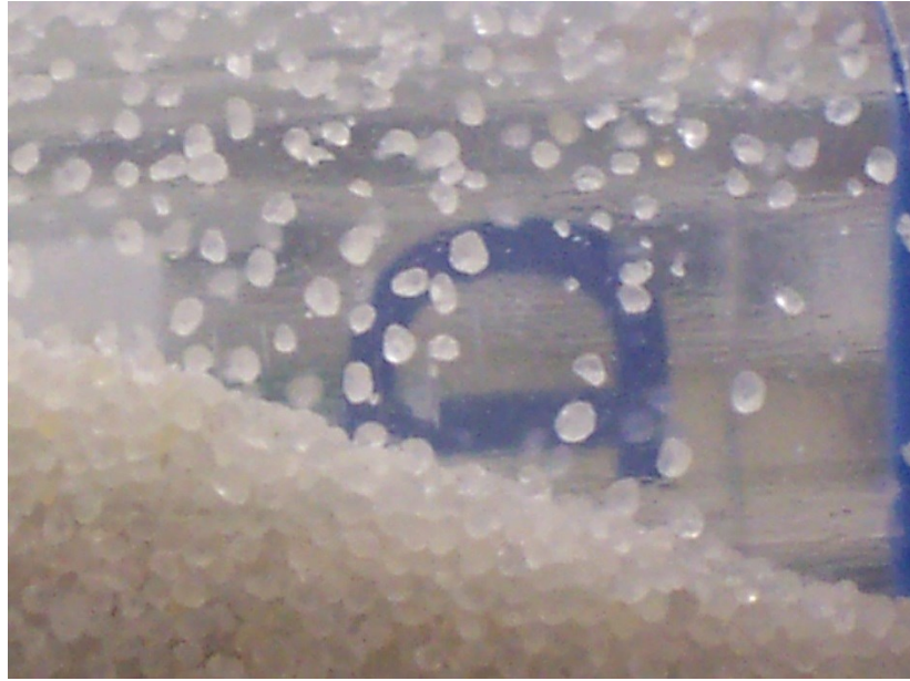
Figure 9: Microscopic image of Ottawa sand
