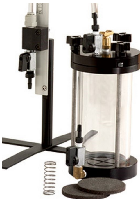
Figure 62: Permeameter for hydrophobic sand
