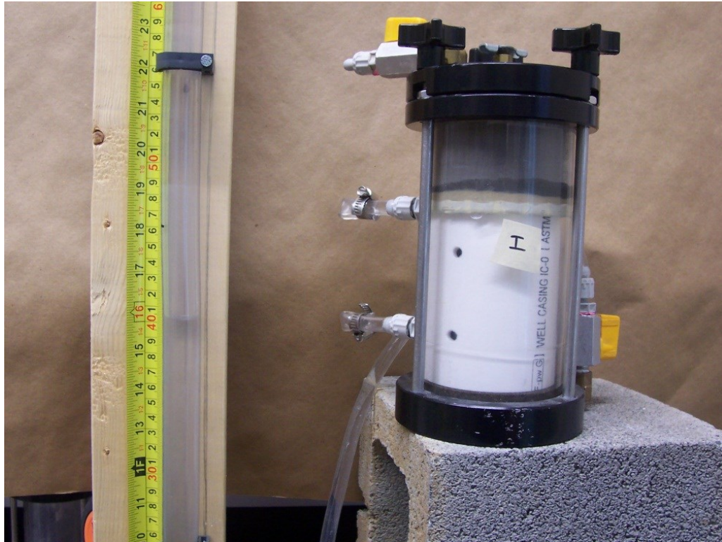
Figure 73: Hydrophilic CFA in standpipe apparatus
