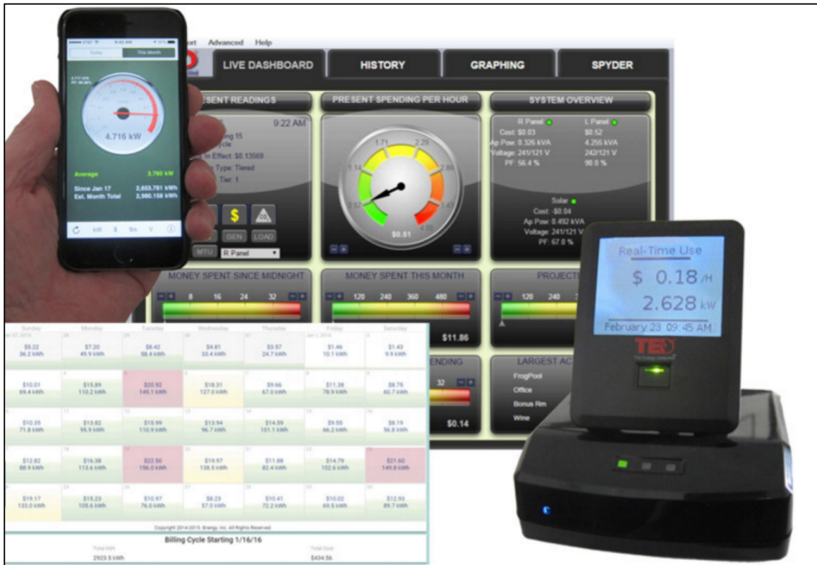
FIGURE: 1.1 A user interface image of the energy detective (TED) pro home [11]
