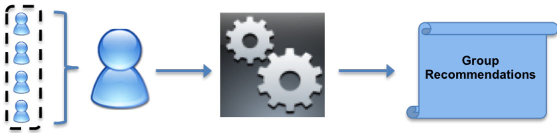
Figure 6: Recommender systems merge user models based on an aggregation algorithm to create a group user model. The group user model is utilized by the filtering technique to generate group recommendations that fit the target model.
