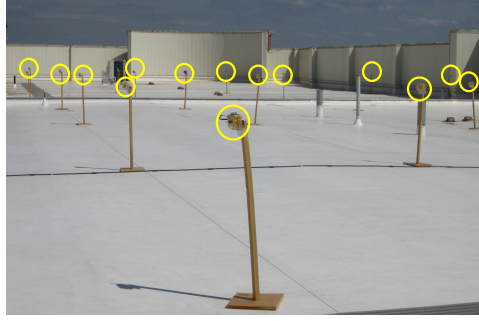
Figure 11.6: A 25-node wireless sensor network testbed.
