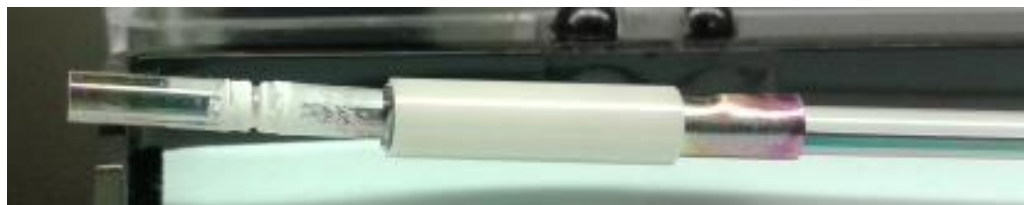
Figure 3.15: The short resonator rod attached to a long 2mm diameter glass rod with a ceramic sleeve. Metal shim was used to fill the gap between sleeve and the 2 glass rods.
