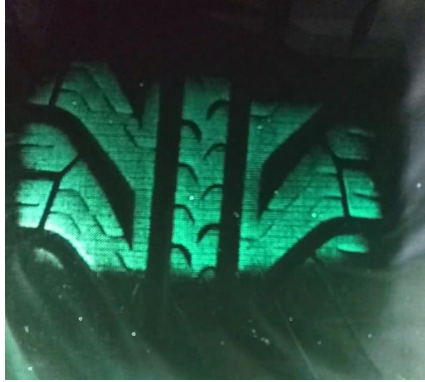
Figure 2.15: Normal load image using FTIR technique at 3^{\circ} of slip angle.
