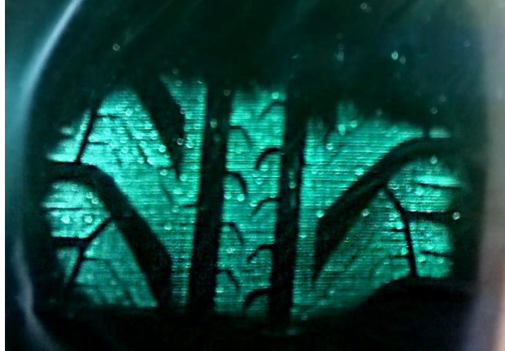
Figure 2.21: Normal load image using FTIR technique at 6^{\circ} of slip angle.
