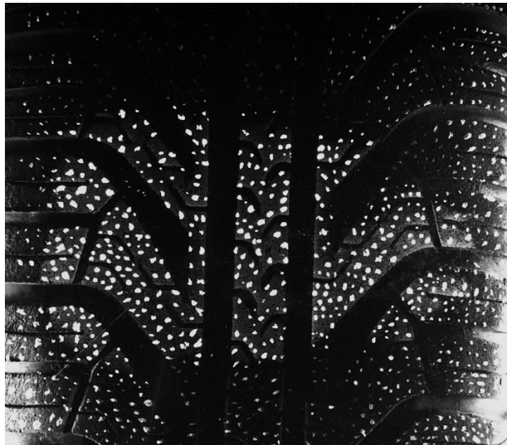
Figure 2.18: Greyscale displacement image using white tread dots on bare glass at 4^{\circ} of slip angle.
