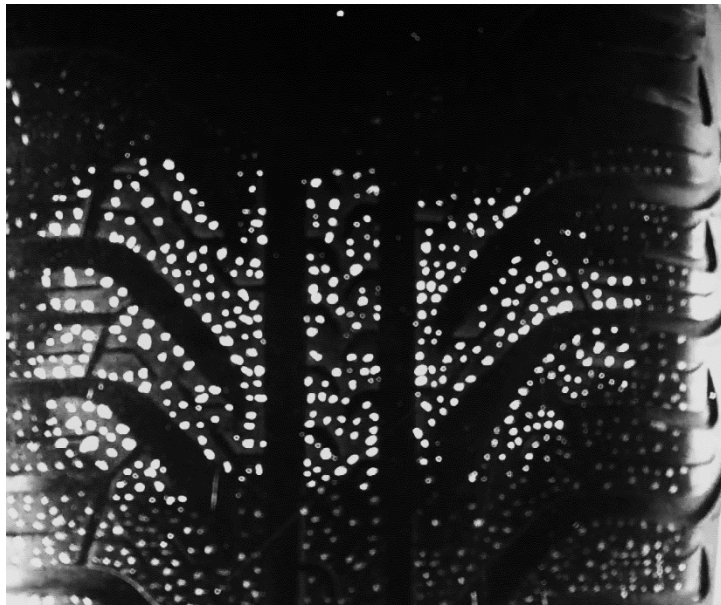
Figure 2.16: Greyscale displacement image using white tread dots on bare glass at 3^{\circ} of slip angle.
