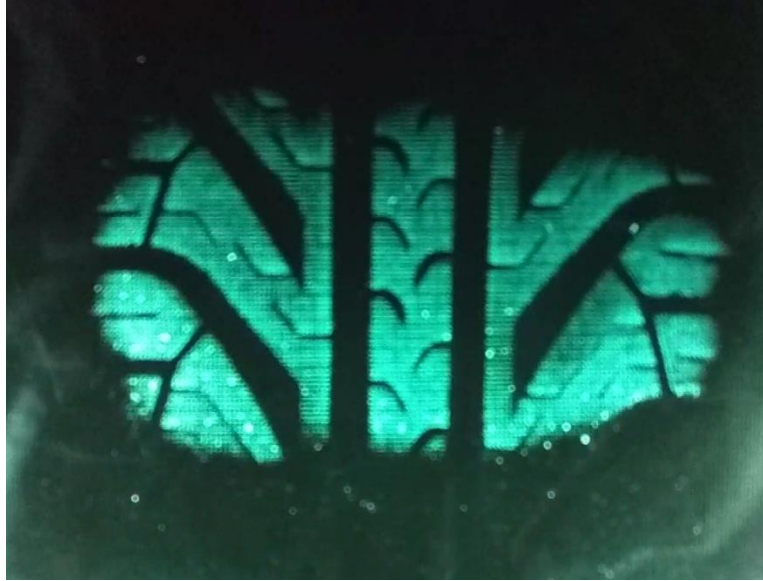
Figure 2.11: Normal load image using FTIR technique at 1^\circ of slip angle.
