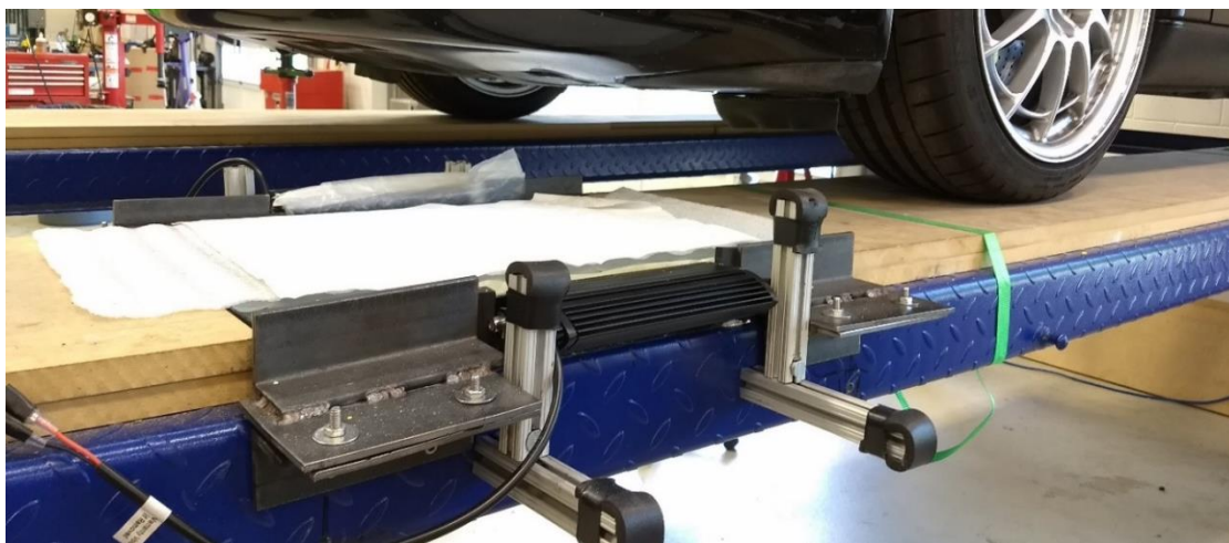
Figure 2.4: High powered LED lights mounted onto a frame to achieve FTIR.
