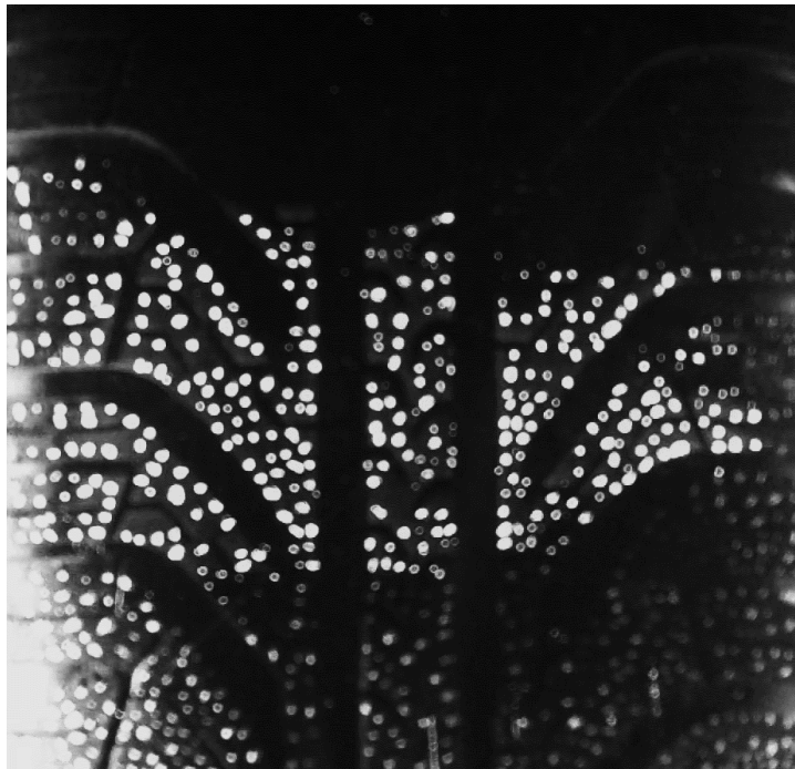
Figure 2.14: Greyscale displacement image using white tread dots on bare glass at 2^{\circ} of slip angle.
