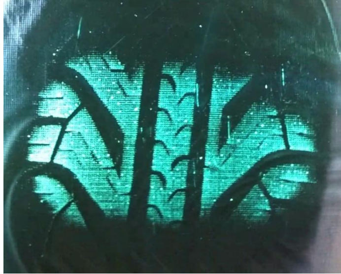
Figure 2.19: Normal load image using FTIR technique at 5^{\circ} of slip angle.
