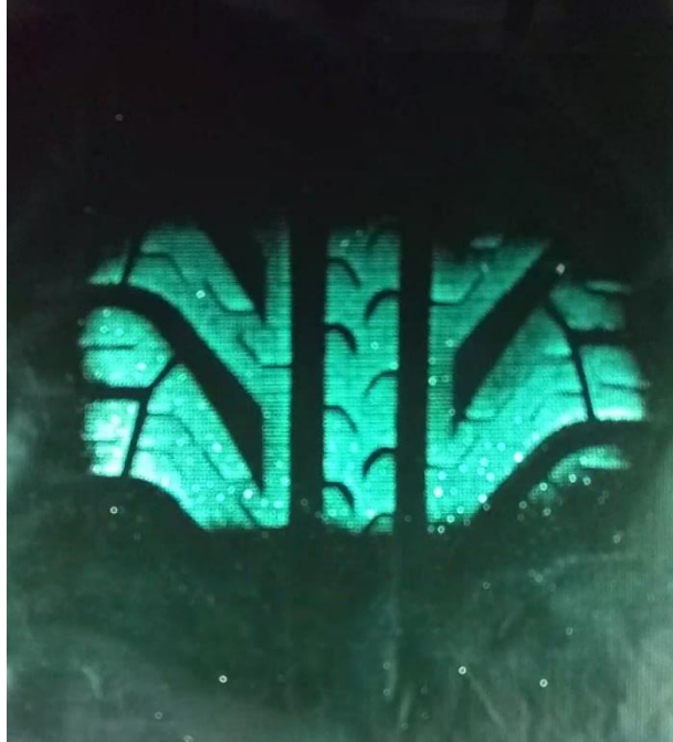
Figure 2.9: Normal load image using FTIR technique at 0^{\circ} of slip angle.
