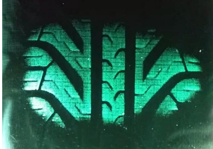
Figure 2.13: Normal load image using FTIR technique at 2^{\circ} of slip angle.
