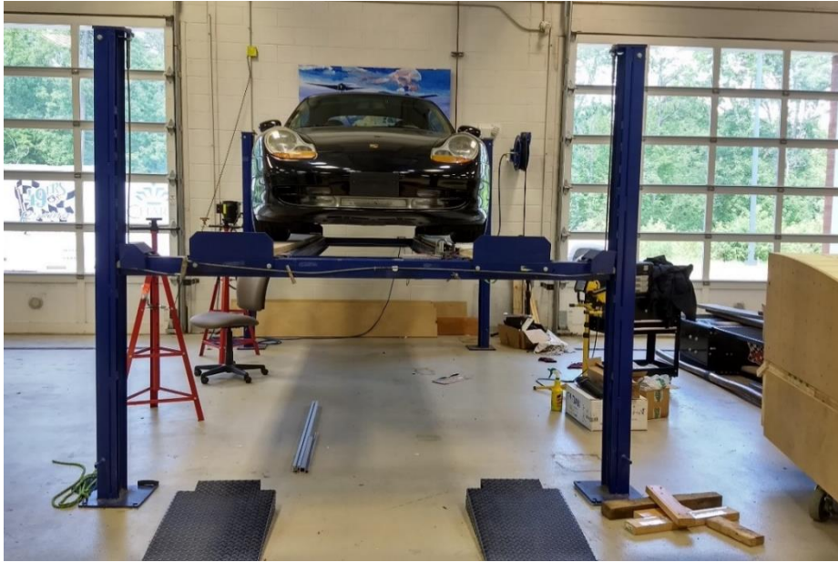
Figure 2.1: Porsche 911 sitting on the modified four-post lift.
