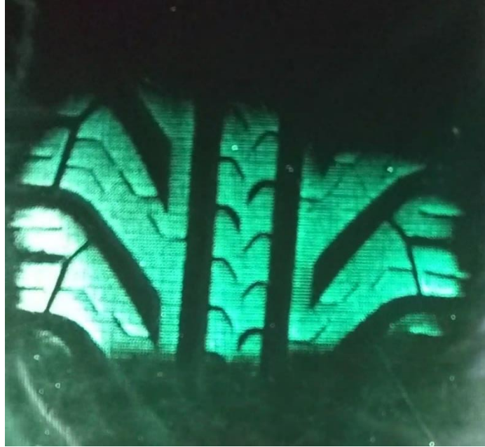
Figure 2.17: Normal load image using FTIR technique at 4^{\circ} of slip angle.
