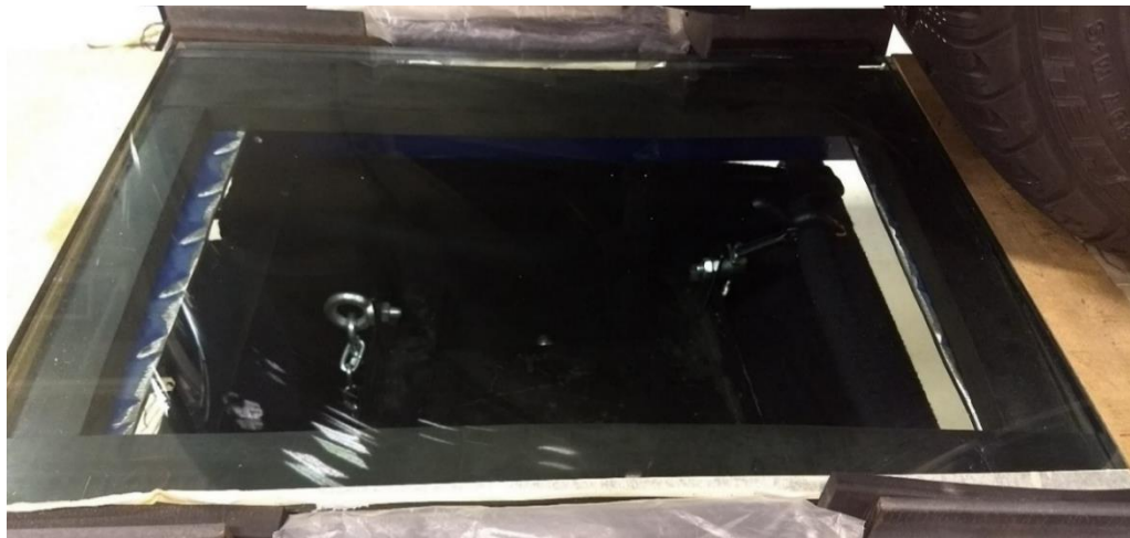
Figure 2.2: 559mm x 407mm x 19mm thick glass panel mounted onto a rubber frame.
