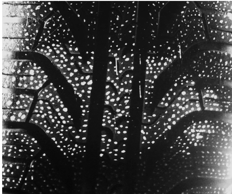
Figure 2.20: Greyscale displacement image using white tread dots on bare glass at 5^{\circ} of slip angle.
